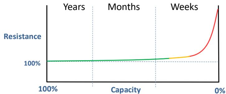
Much the optimum solution in Ohmic testing therefore is continuous monitoring and trending of measured parameters to detect small changes before larger ones.
